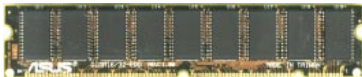
ECC EDO DIMM (9 chips) 72bits
